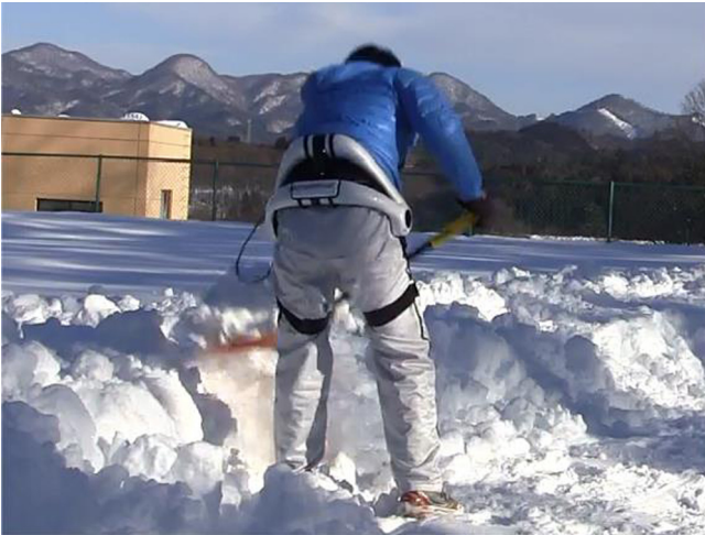
Fig. 2. A study participant shoveling snow using the HAL for Care SupportCare Support.
